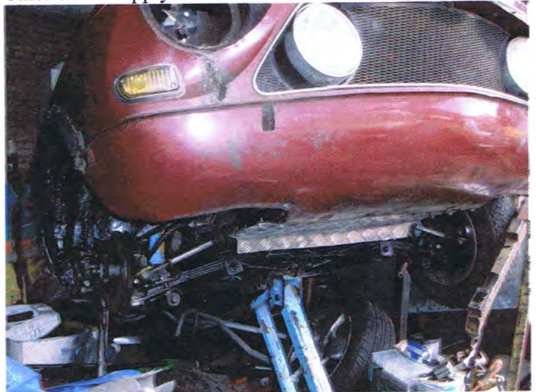
Area below radiator now has removable section in thick alloy as access to hoses etc. down there.
