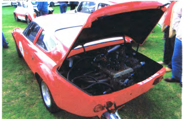
Abarth SIMCA 2000 showing off its twin cam,
