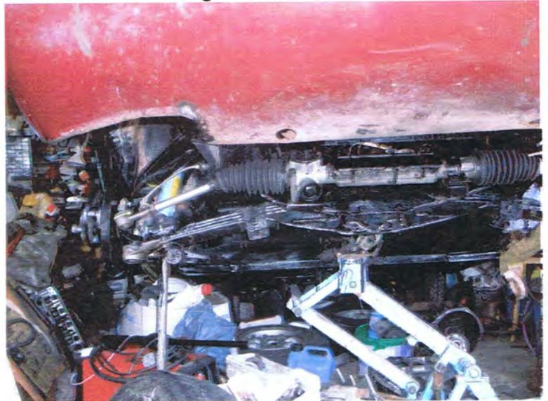
Rack from late SIMCA 1000 saloon fitted with Alpine trackrods and original 1000 ends.
