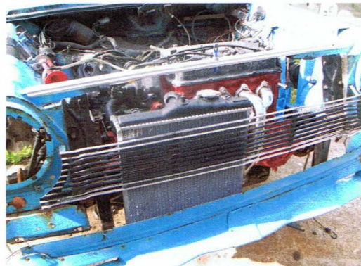
Checking everything fits inside the front, prior to new panel being fitted
