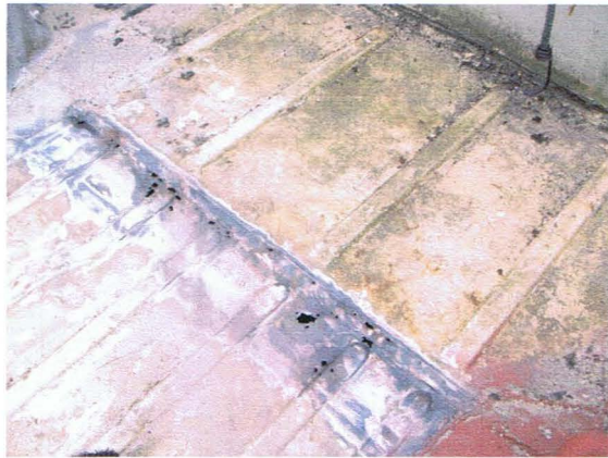
Holey area on joint of floor sections and rear end of pickup bed that was rusted / worn through ...
