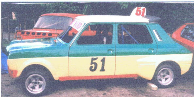
Mick's 1000 built for the Buxton 1600 FWD 'Hot Rod' class.. Note Rear arch extensions made from Bagheera wings..
