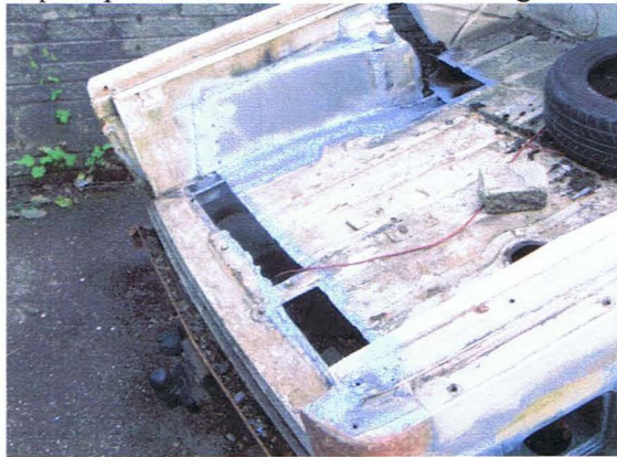
Holey area on joint of floor sections and rear end of pickup bed that was rusted / worn through ...
