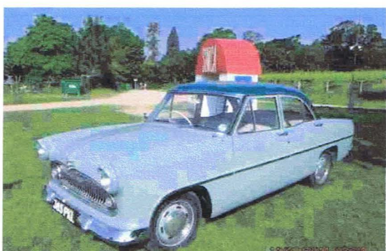
Rare in RHD form, the Ariane.... The body from the V8 Vedette with 4 cylinder 1290cc engine from the Aronde.....
